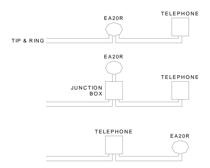
Figure 3 - Wiring Alternatives
